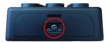
Now insert 4 x AAA batteries, push the battery compartment back into the housing and screw it tight. To test the functionality of the keypad, check whether the green status LED (top right) flashes when a button is pressed.
