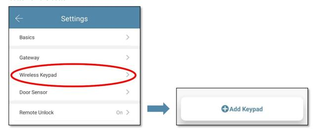
In order for the wireless keypad to be recognised by the mobile phone, the **configuration mode** must be **activated**. This is the case when the **LED** (top right)on the device **flashes green**. If so, click on "**Next**".
